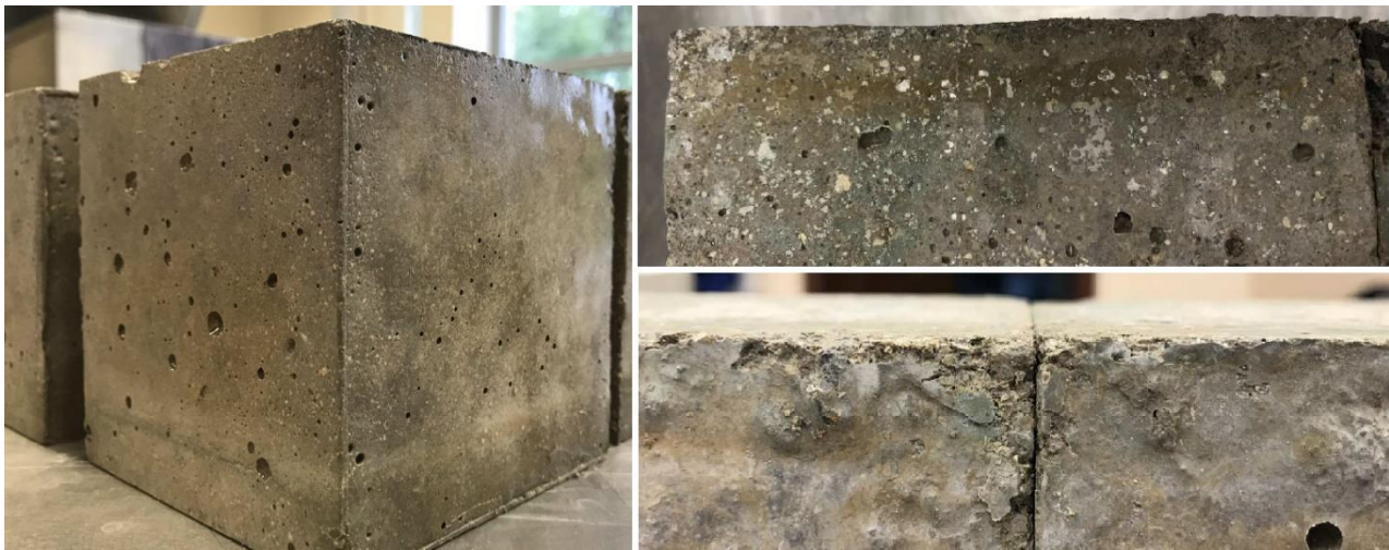
Figure 12. Surfaces of specimens after freezing/thawing cycles.
