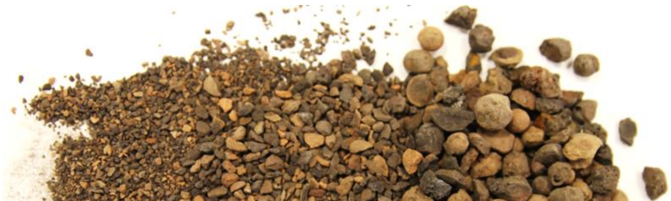
Figure 1. SFA aggregate divided by fractions (from left: 0/2 mm; 1/4 mm and 4/8 mm).
