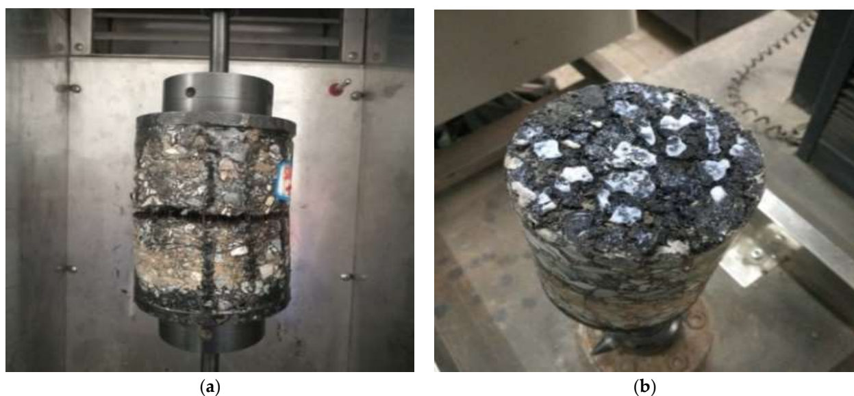
Figure 10. Direct tensile test of the interlayer bond: (a) the direct tensile failure; (b) the detachment between the drawing head and the specimen.
