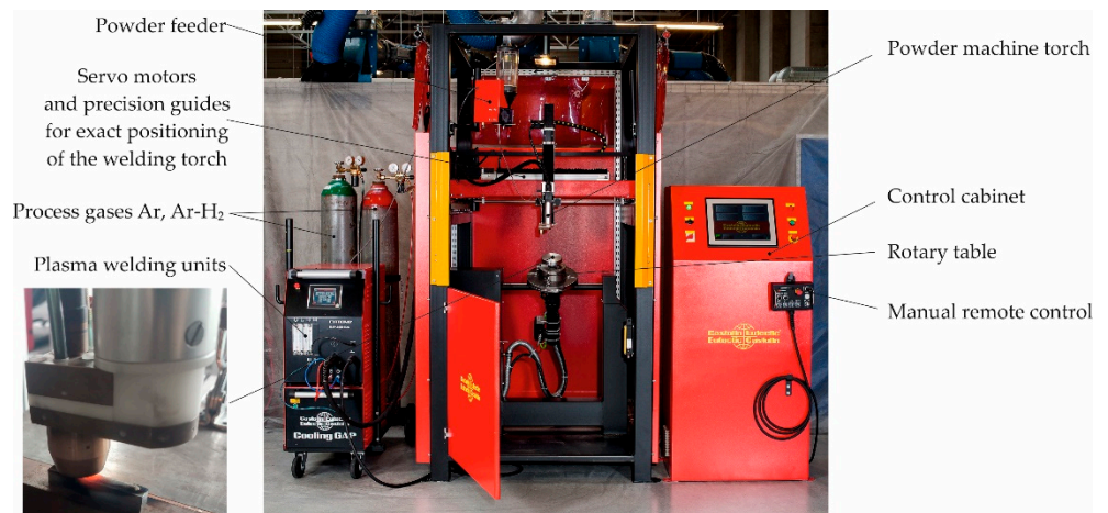
Figure 3. Gap automated unit robotic coating system.
