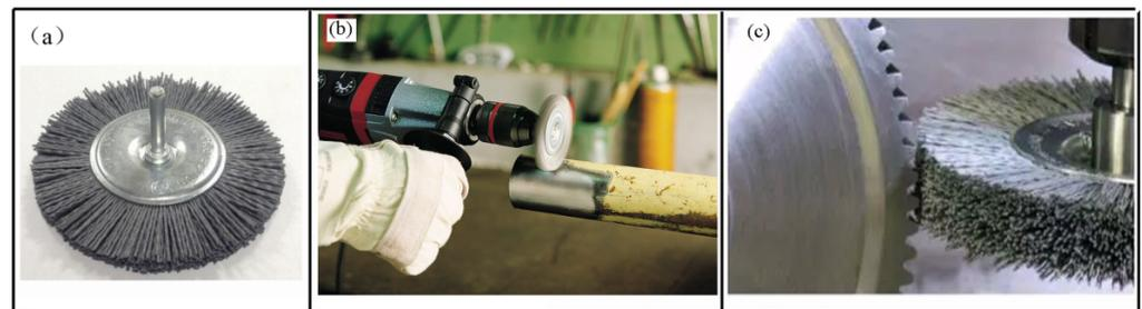
**Figure 1.** Abrasive filament brush (a); brush derusting (b); and grinding gear (c).
