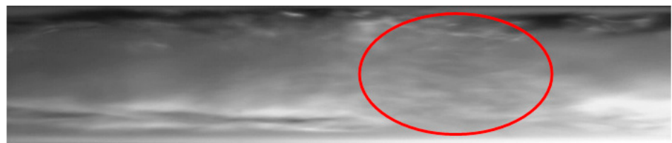
Figure 12. Froth formation in annular-wave flow at high speeds of both phases during condensation of Novec649 refrigerant in a minichannel with internal diameter d_h = 2.0 mm ( G = 1796 kg/m 2 s; x = 0.01 ; \phi = 0.5 ; t_s = 54 °C).
