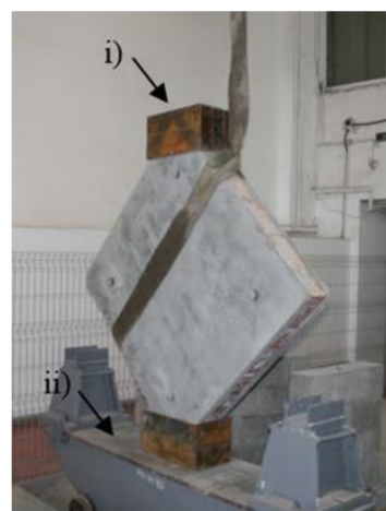
Figure 10. Specimen positioned on the transportation carriage: (i) loading shoe and (ii) transportation carriage.
