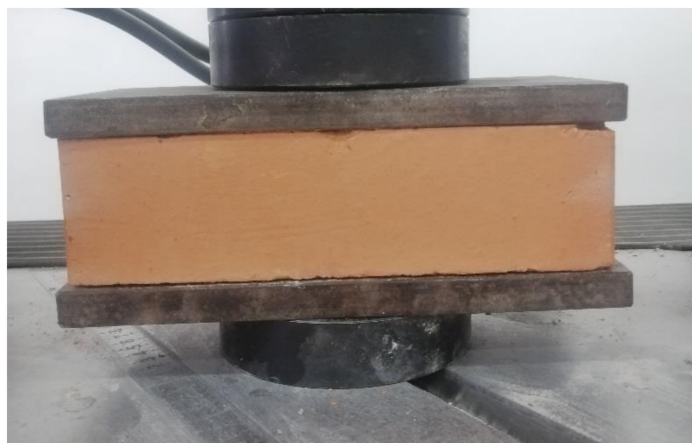
Figure 3. Brick unit tested in compression using a WAW 600 Universal Testing Machine.
