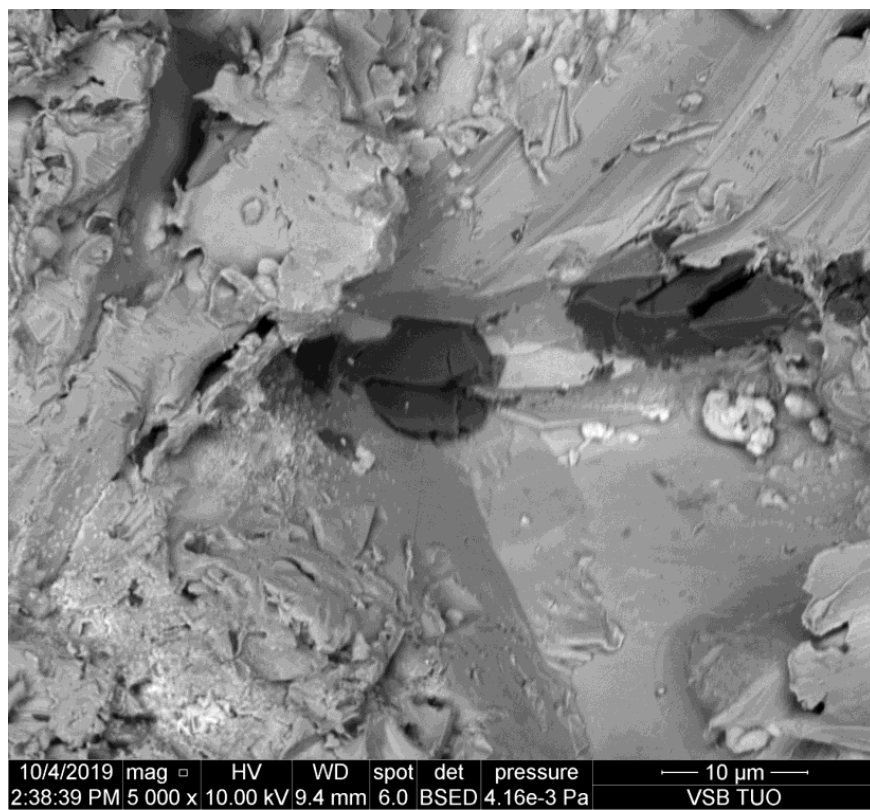
Figure 3. Abrasive particles observed on the sidewall of the kerf made in brass.
