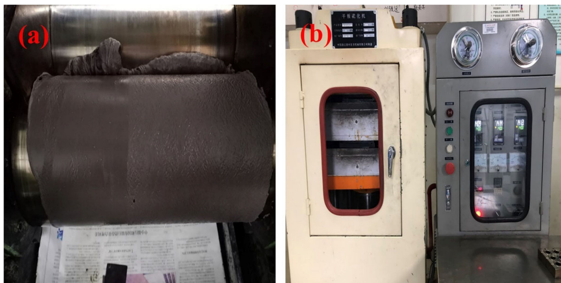
Figure 1. (a) the preparation process of various MPU/EUG composites by using an open mill; (b) the vulcanizing instrument used in this work.
