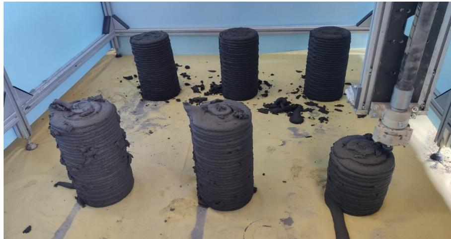
**Figure 5.** Printing of concrete columns.
