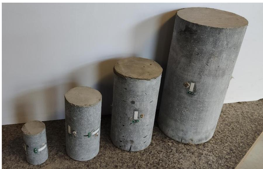
**Figure 7.** Core drilled specimens with strain gauges installed on them.
