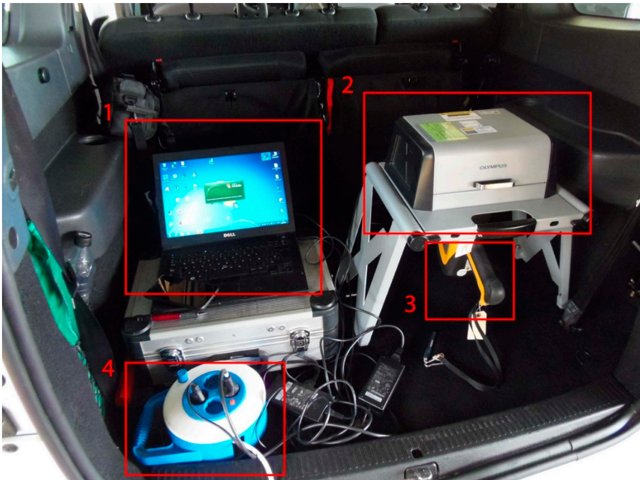
Figure 2. Experimental setup for in-situ chloride analysis. (1) Laptop computer; (2) Workbench; (3) Handheld X-ray fluorescence analyser (hXRF) analyser; (4) External generator (photo taken by S. Chinchón-Payá).
