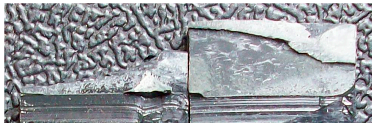
Figure 15. Fracture surface of a specimen pretreated with plasma using D = 5 mm and v = 100 mm/s.
