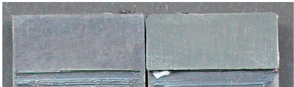
Figure 9. Fracture surface of the abraded specimen subjected to the quasi-static tensile test.
