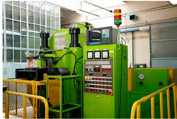
Figure 5. Device for high pressure spark plasma sintering [133].
