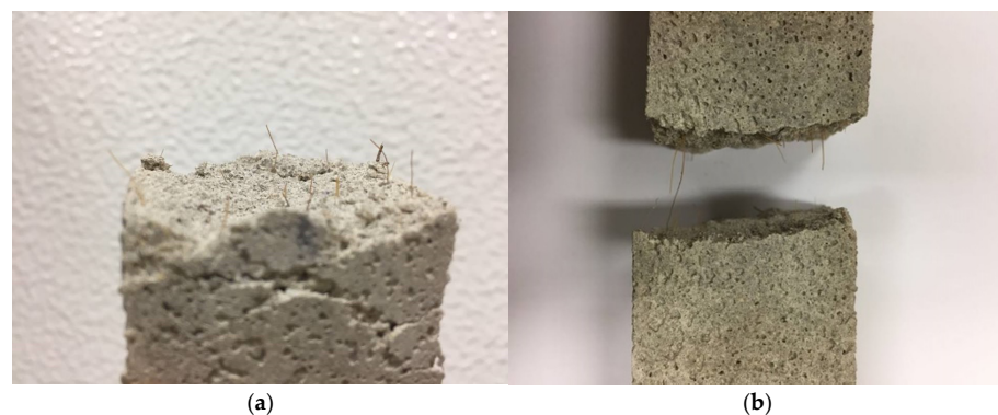
Figure 10. Coir fiber-reinforced cement-based mortars specimens after (a) compressive strength test and (b) flexural strength test.
