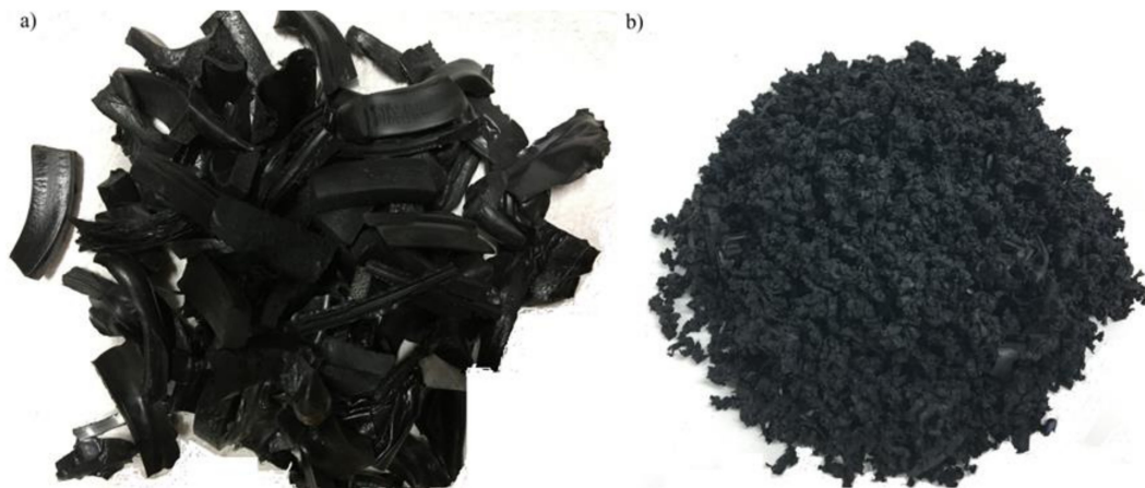
Figure 1. Production waste from the production process of car floor mats: (a) initially crushed material; (b) material crushed to 2–8 mm fraction.
