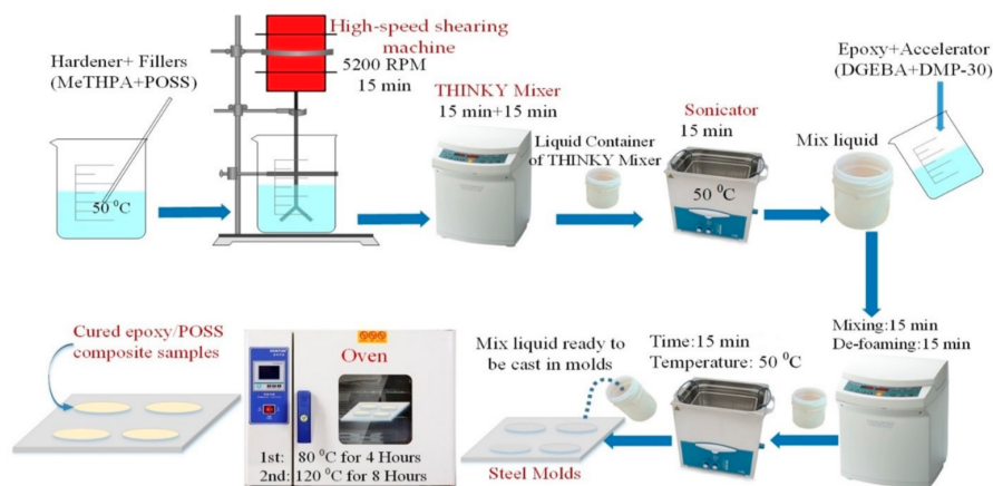
Figure 1. Fabrication process of epoxy/POSS nanocomposite samples.
