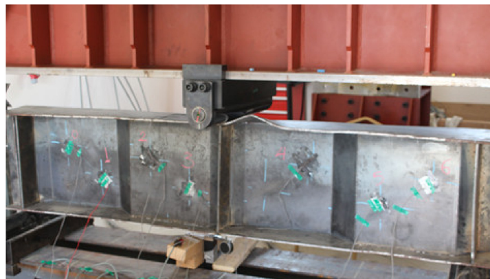
Figure 9. Failure mode of specimen CW35IFWL.
