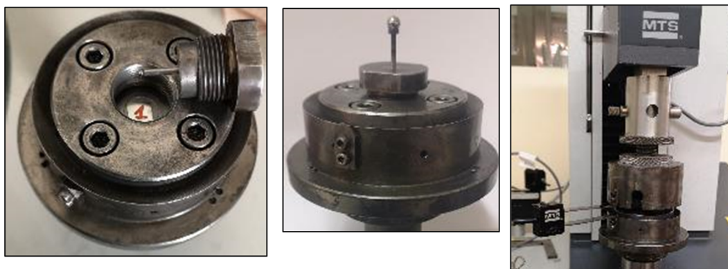
Figure 9. Specimen 1 placed in the SIMUMECAMAT SPT testing device (left). Punch rod (middle). SPT testing machine (right).
