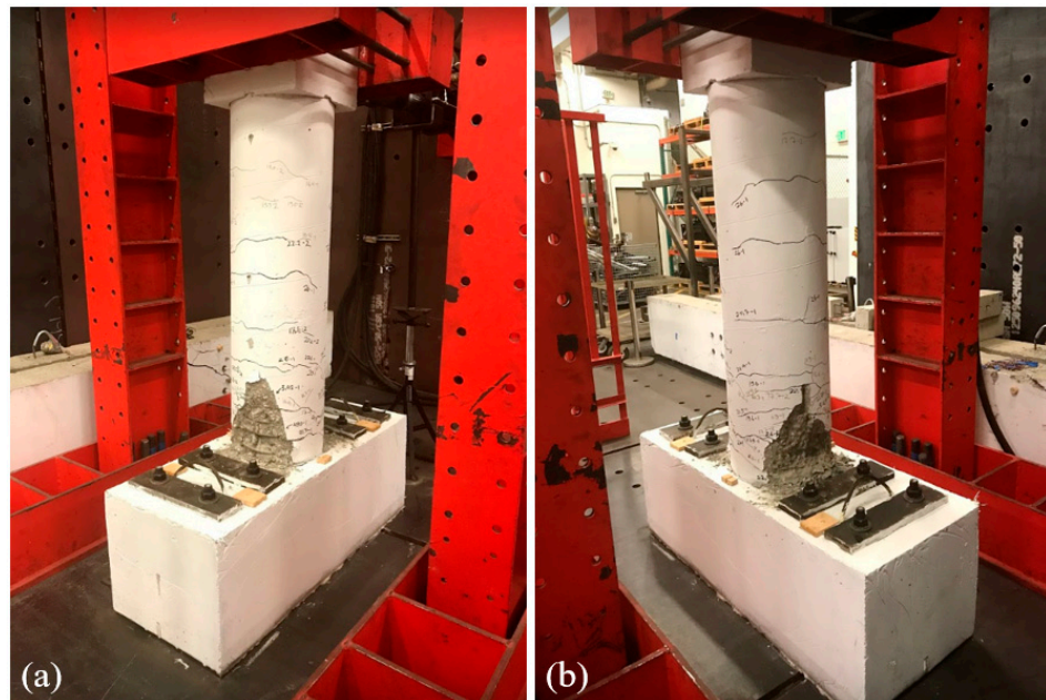
Figure 7. Column condition after testing (a) East and (b) West view.
