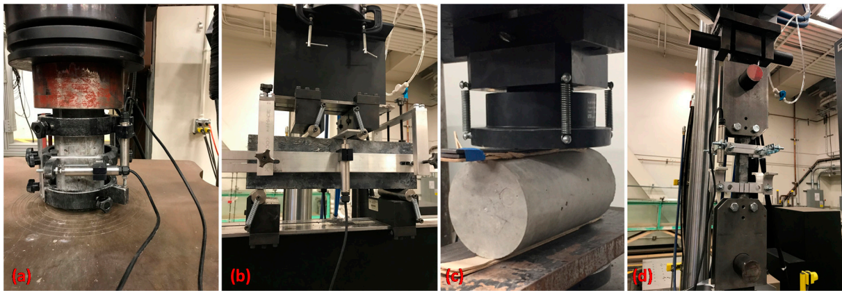
Figure 3. Material tests (a) compression, (b) flexure, (c) split tension, and (d) uniaxial tension on NSC and UHPC. Note that uniaxial tension tests were only performed on UHPC samples.
