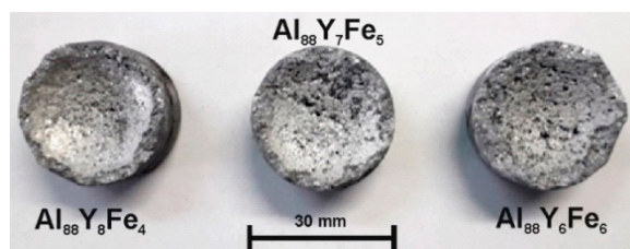
Figure 1. External morphology of \text{Al}_{88}\text{Y}_8\text{Fe}_4 , \text{Al}_{88}\text{Y}_7\text{Fe}_5 , and \text{Al}_{88}\text{Y}_6\text{Fe}_6 alloys in the form of ingots.
