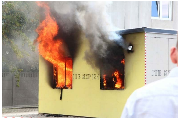
Figure 1. View of flames escaping from a room involved in a fully developed standard fire, during a field test. (Author: E. Kotwica).
