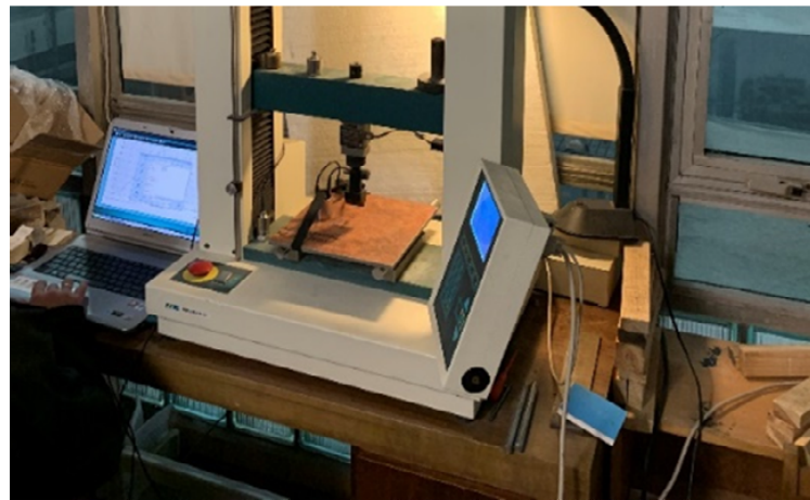
Figure 10. Three-point bending flexural testing machine.
