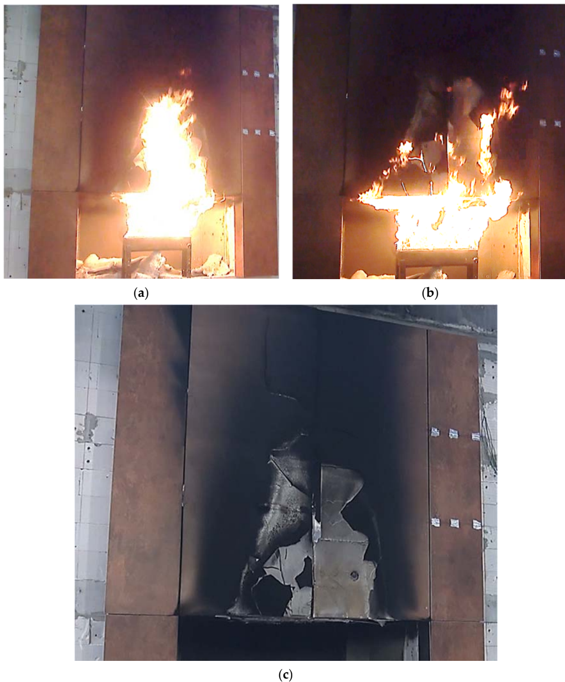
Figure 7. View of the large-scale facade model in the subsequent minutes of the test: (a) approximately 40'00"—high cladding degradation; (b) approximately 55'00"—more elements are falling off; (c) view of facade cladding after testing.
