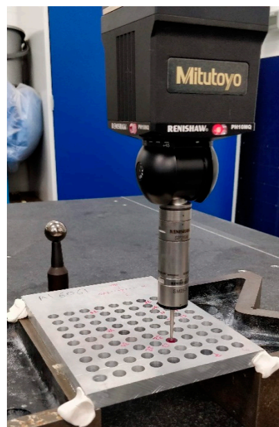
Figure 2. Al6061 workpiece setup inside the CMM machine.
