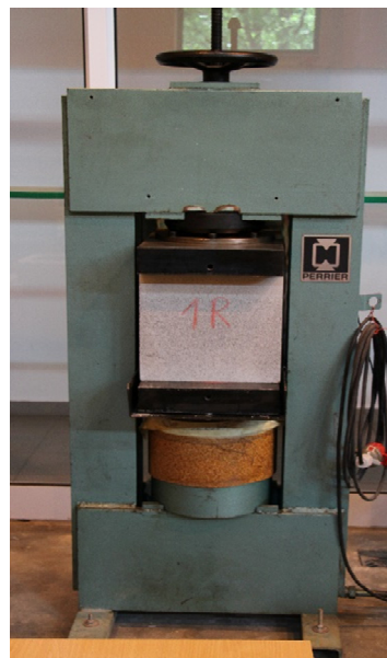
Figure 8. Course of strength testing—compression of a block in a hydraulic press.
