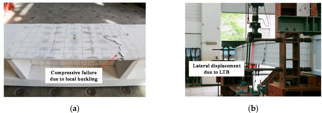
Figure 2. Examples of buckling failure in concrete slender members: (a) local buckling of thin-walled ultra-high performance concrete (UHPC) flanges (a test specimen conducted from reference [22]) and (b) lateral-torsional buckling (LTB) of slender UHPC I-girder (test specimen conducted from reference [21]).
