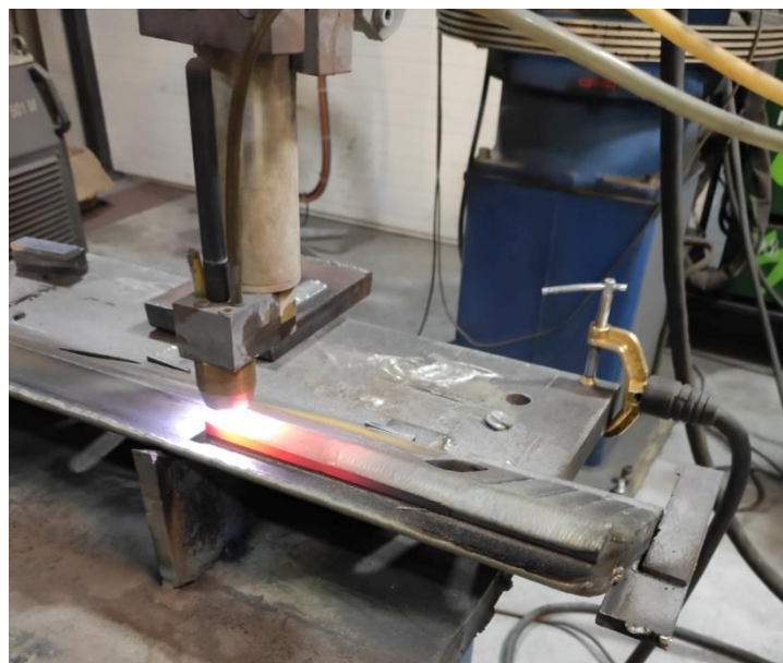
Figure 2. View of the powder plasma transferred arc welding (PPTAW) processes.
