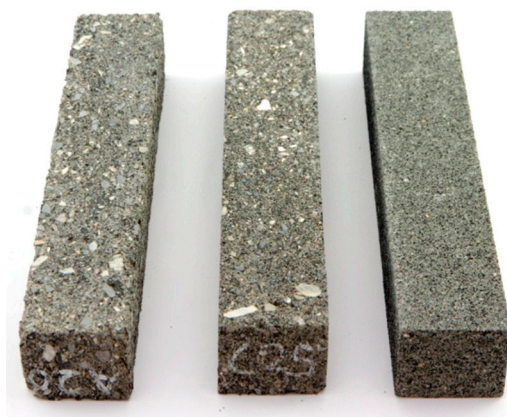
Figure 2. Beams 380 mm × 63 mm × 50 mm of ACC with “B” mortar, and “B” CSR mortar alone for testing the stiffness modulus using 4PB-PR method.
