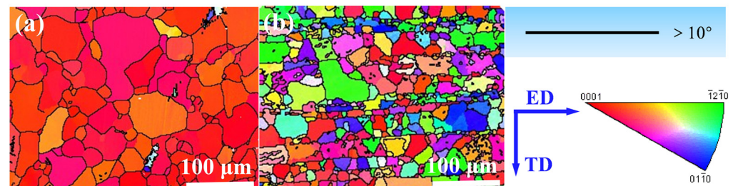
Figure 6. The IPFs results of bulk Mg and 0.5 wt.% CNTs/Mg composites on the ED-TD plane. (a) bulk Mg; (b) CNTs/Mg composites.
