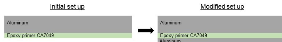
Figure 13. Difference in material set up after the addition of aluminum tape in the FE model.
