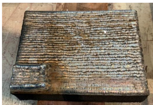
Figure 2. Plain plate welded by manual TIG welding technique.
