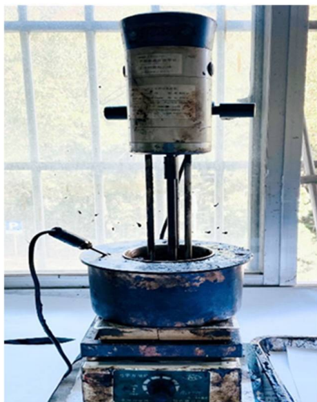
Figure 2. High-speed shear agitator for BRA-MA preparation.
