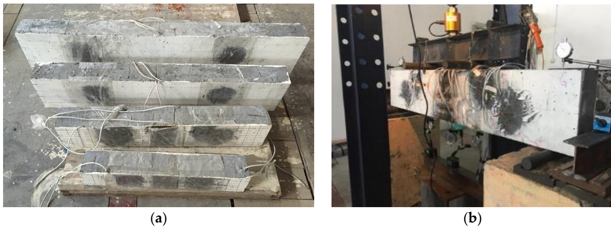
Figure 2. Beam specimens and the loading equipment. (a) Beam specimens with different sizes. (b) Loading equipment of four-bending test.
