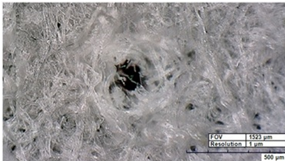
Figure 1. An exemplary view of a filter paper with Na solution after 3 laser shots.
