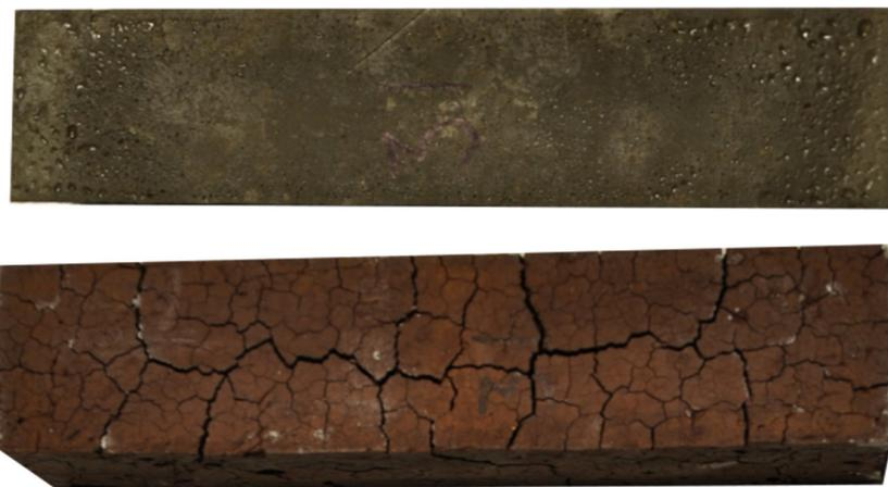
**Figure 5.** Top view of sample 31: up, before heat exposure; down, after heat exposure.
