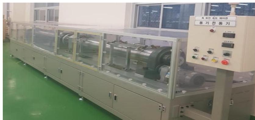
Figure 5. Photo of the experimental setup for electrical pitting prevention device.
