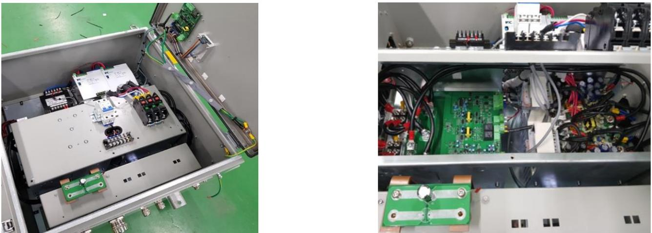
**Figure 2.** Photo of the electrical pitting prevention device.
