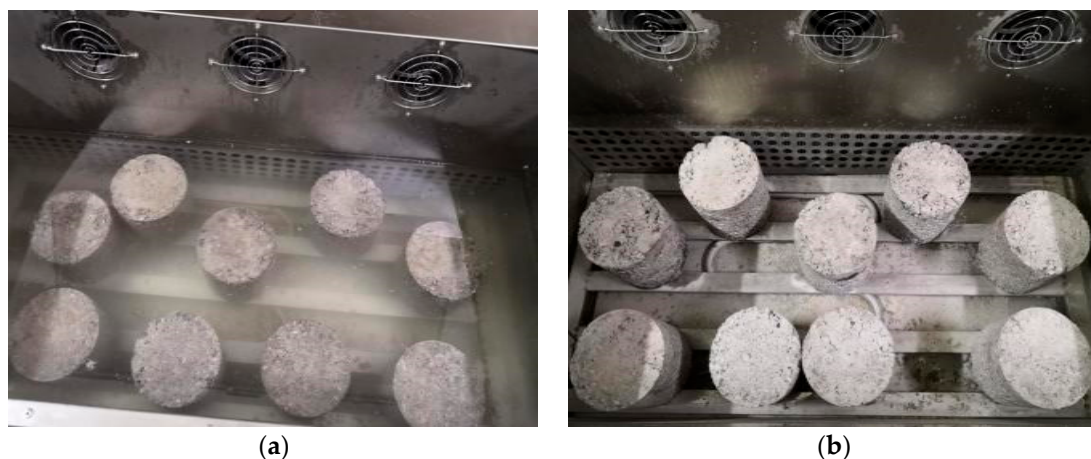
Figure 9. Freezing and thawing process: (a) Fused specimen; (b) Frozen test piece.
