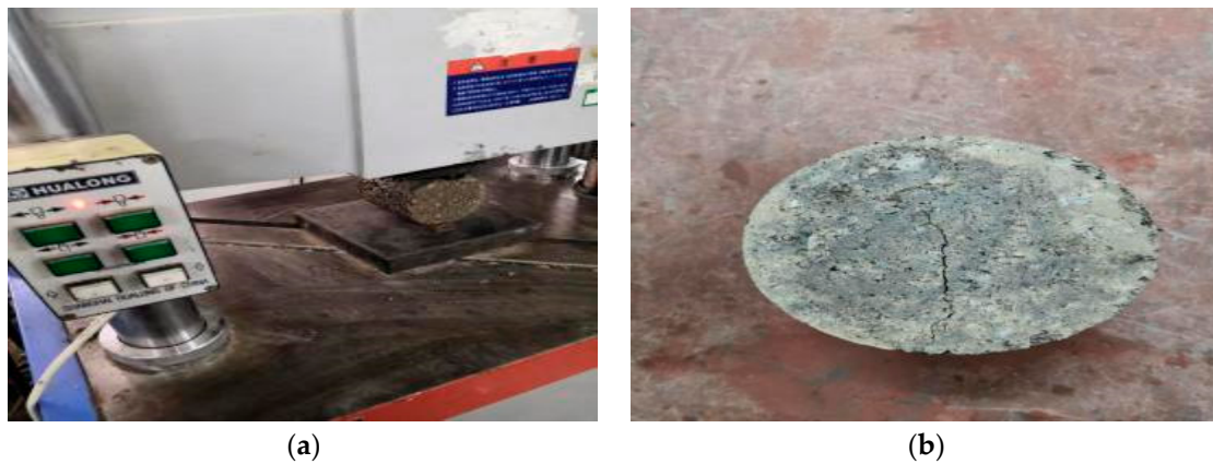
Figure 6. Splitting strength test: (a) In test; (b) After test.
