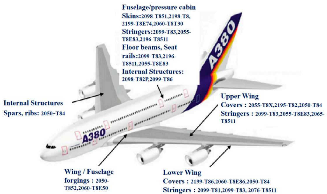
Figure 2. Typical uses of aluminum alloys in an A380 aircraft [15].
