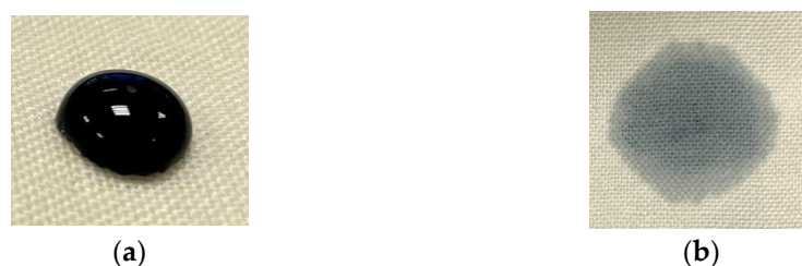
Figure 5. Photographs of “conductive acid dye” PEDOT: PSS and water (1:1) solution drop (see Table 3) on (a) untreated and (b) plasma-treated wool.
