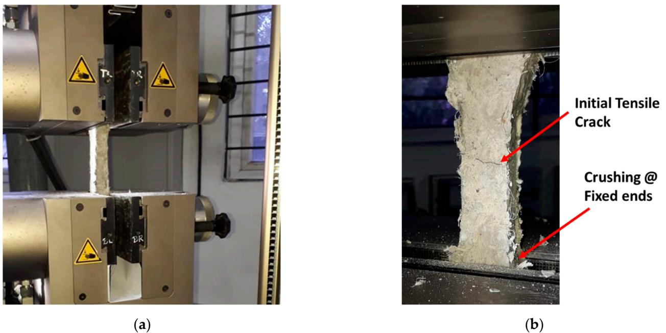
Figure 3. Tensile testing of ECC coupons. (a) Test Setup, (b) Failure Mode.
