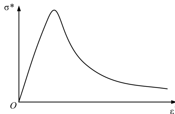
Figure 2. Uniaxial tensile stress–strain curve.
