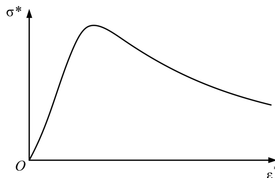
Figure 3. Uniaxial compressive stress–strain curve.
