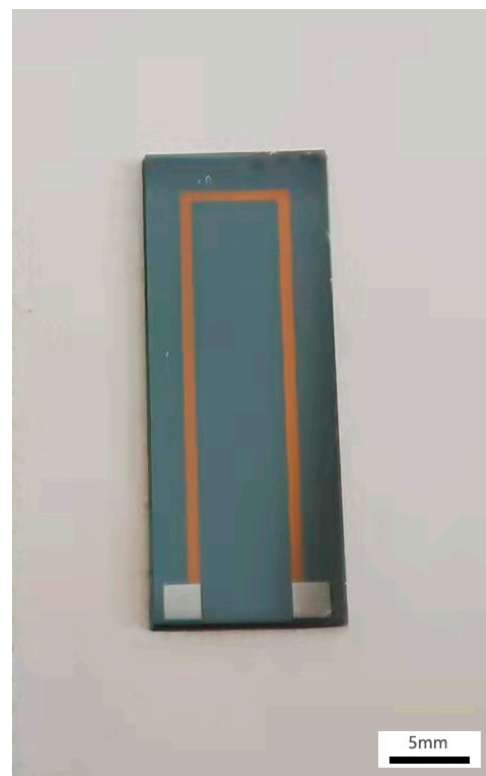
Figure 2. The fabricated TFTC by MEMS process.
