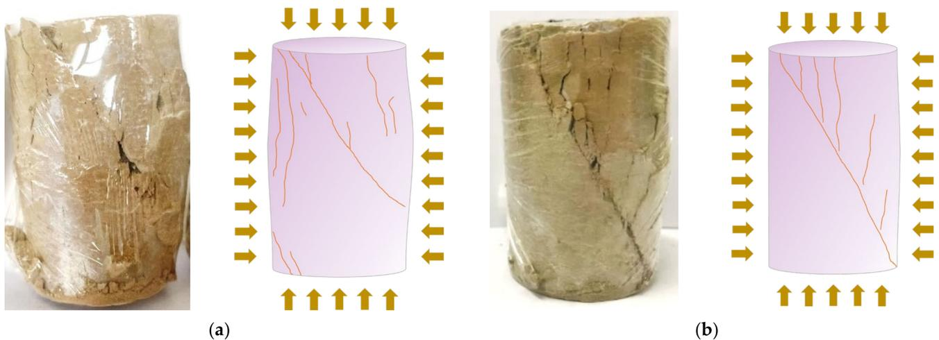
**Figure 8.** The failure of two specimens under confining pressure of 0.9 MPa: (a) LC-0 specimen group and (b) LC-12 specimen group.
