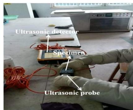
Figure 2. The ultrasonic velocity test process.
