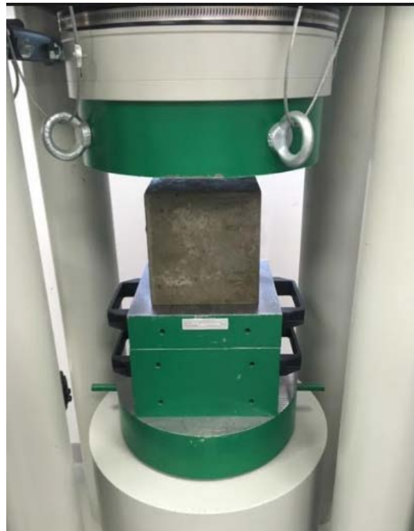
Figure 2. Sample during compressive strength test.
