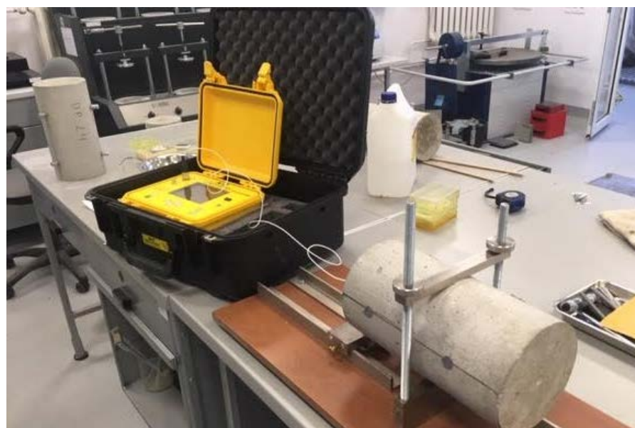
Figure 5. Resonance testing of the modulus of elasticity.
