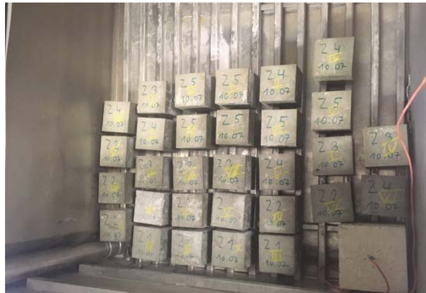
Figure 4. Samples prepared for frost resistance testing.
