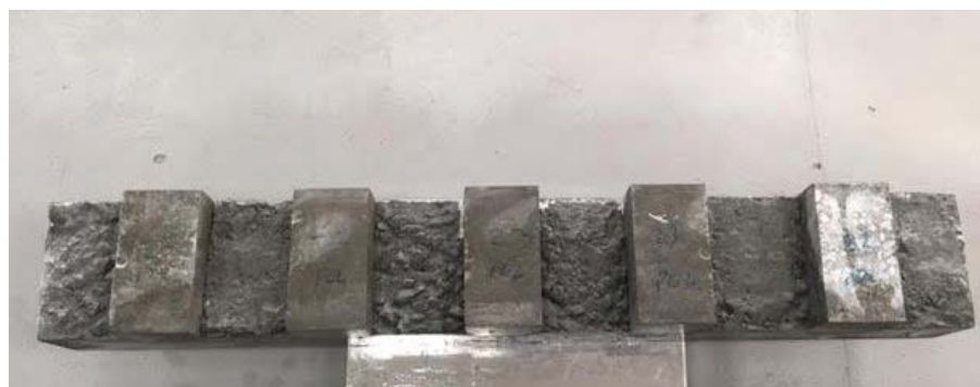
Figure 13. Prepared sample for bending strength testing.
