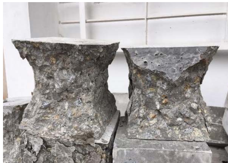
Figure 3. Concrete samples after compressive strength test.
