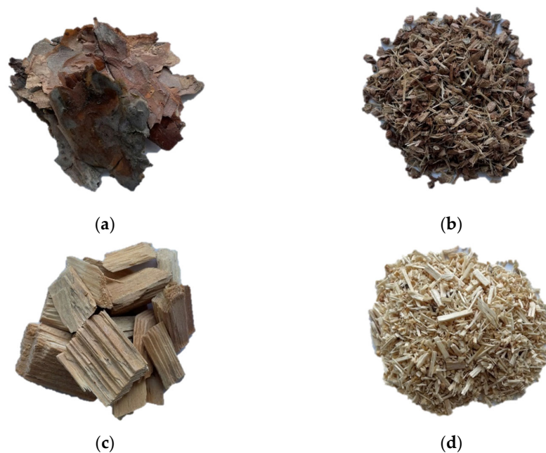
Figure 1. Materials used for the production of boards: (a) bark particles before grinding; (b) bark particles after grinding; (c) wood chips; (d) sawdust.
