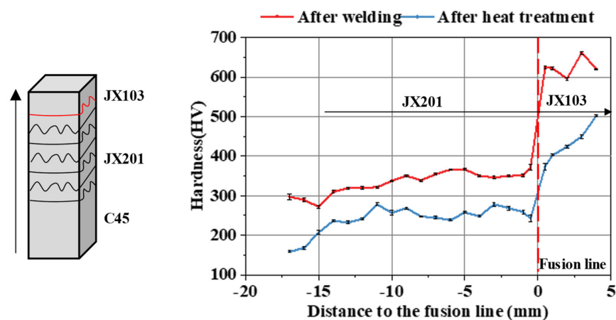
Figure 4. Microhardness distribution difference after welding and heat treatment (along the building direction).
