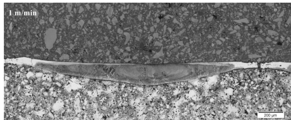
Figure 7. Cross-section of the entire alloyed zone for sample 1.
