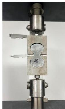
**Figure 4.** Steel fiber pullout test.
