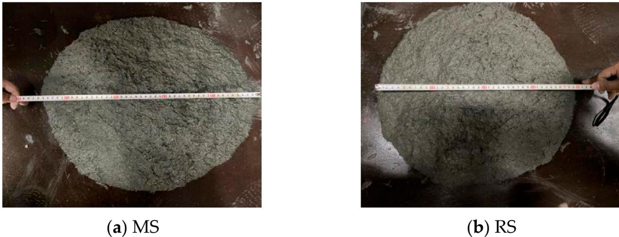
Figure 2. Concrete slump spread test.
