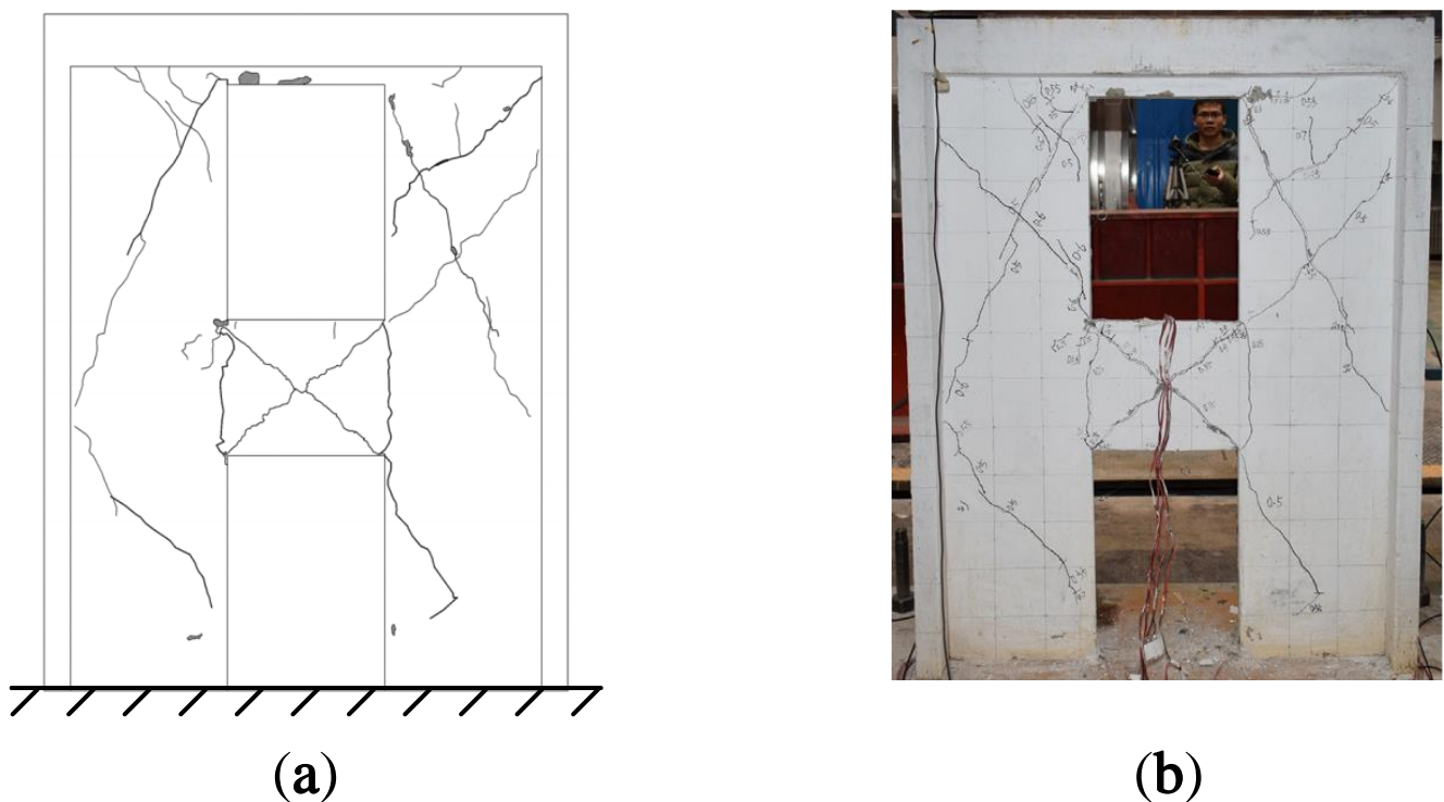
Figure 5. (a) crack diagram; (b) failure mode of A2 [19].
