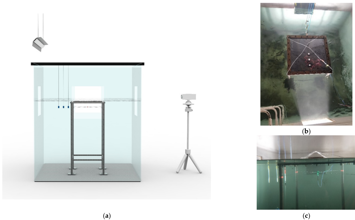
Figure 2. Overview of underwater explosion tests. (a) 3D view of water tank, specimen, and instruments. (b) Top view of specimen. (c) Front view of specimen.
