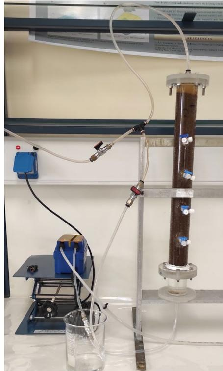
**Figure 1.** The Plexiglas column used for the experimental setup.
