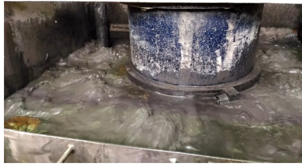
Figure 10. Removal of underburnt by flotation.
